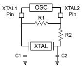
R2 functions as a current limiting resistor to the crystal, and also as an oscillation stabilizer in the presence of perturbations induced by moisture, component variations, or other factors.
